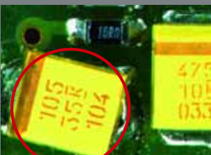
Placement defect: Tantalum capacitor
