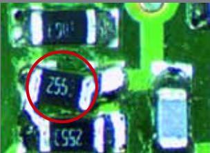
SMD resistor with faulty positioning
