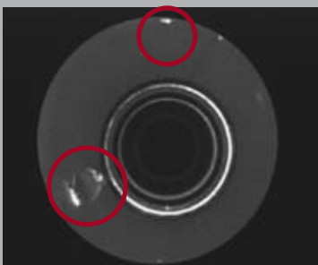
Cylinder interior: Surface defect
