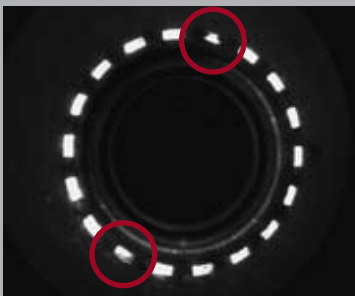
Cylinder interior: Lammellae with defect
