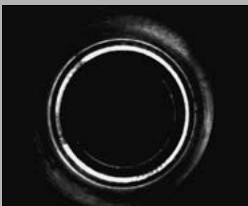
Cylinder interior: Quality control of a seal
