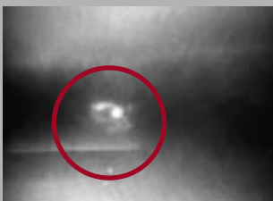
Electrode fusion; insufficient penetration and pores
