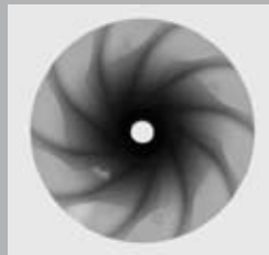
2-D X-ray image, casting defects
