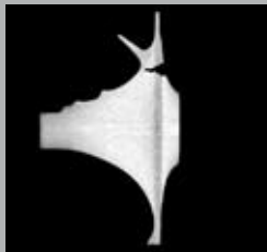
Non-destructive 3-D slice through a casting defect
