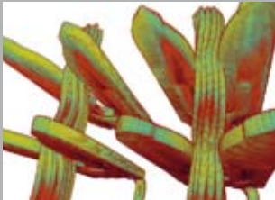
Clamping joints, 3-D volume reconstruction
