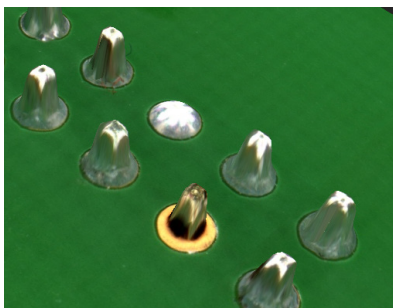
Insufficient wetting (front) and missing pin (back)
