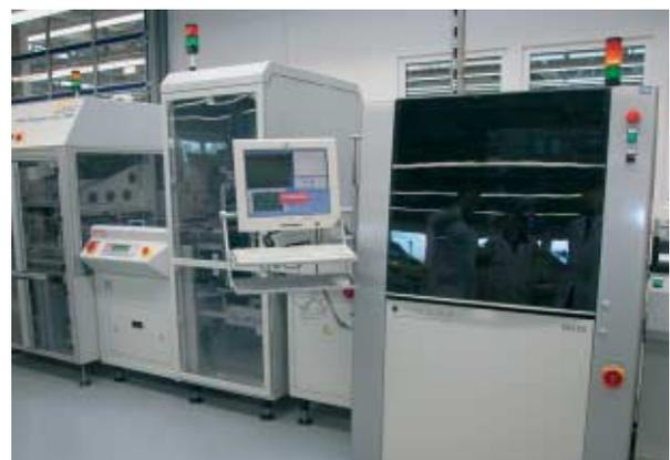
Inspection of lead-free solder joints with the Viscom S6055
