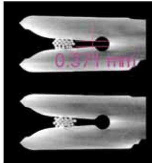
Distance measurement in a μCT-reconstructed contact level of a crimp contact non-destructive 3-D slice
