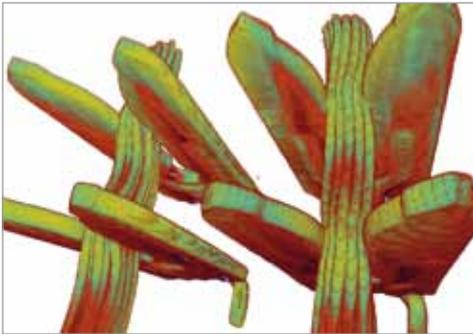
μCT reconstruction of wire bundling in crimped connections
