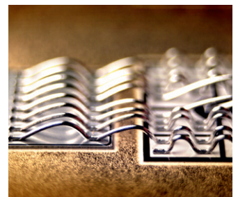
Defect detection on multiwire connections and multiple loops
