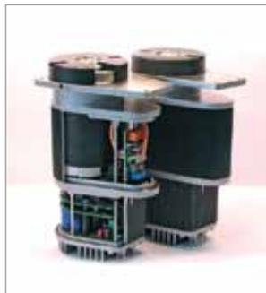
Servo unit with internal electronics
