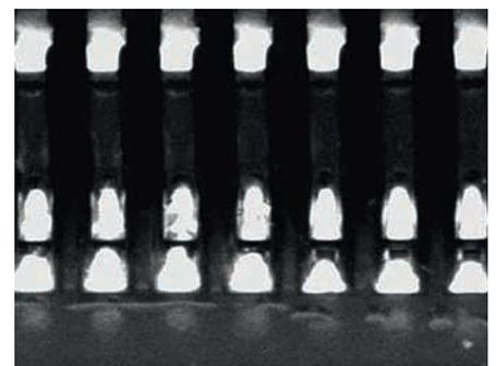
Defects in the angled view with Scheimpflug of all visible solder joints including gull-wing ICs, optical character recognition, data matrix code reading, straightforward recognition of certain polarity marks, high throughput, reasonable costs, and relatively few problems resulting from shadowing. There are many solutions for
