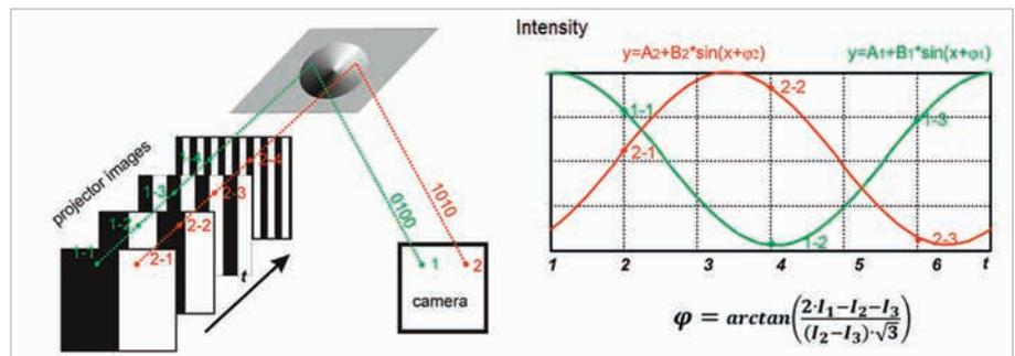
The structured light projection principle
