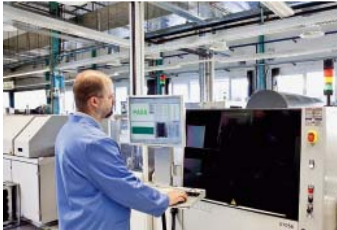
Viscom AOI/AXI combination X7056
