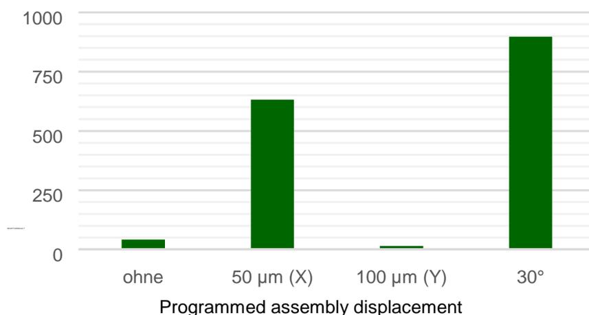
*Image 12: Tombstones occur primarily when the component is horizontally displaced and rotated.*
