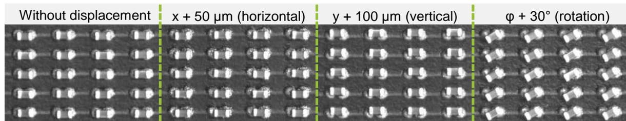
*Image 3: Four positions were considered in the assembly with 01005 components (depiction of the reflow soldering process as example).*
