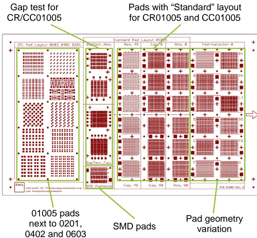
*Image 1: The top side of the printed circuit board permitted a number of tests.*
