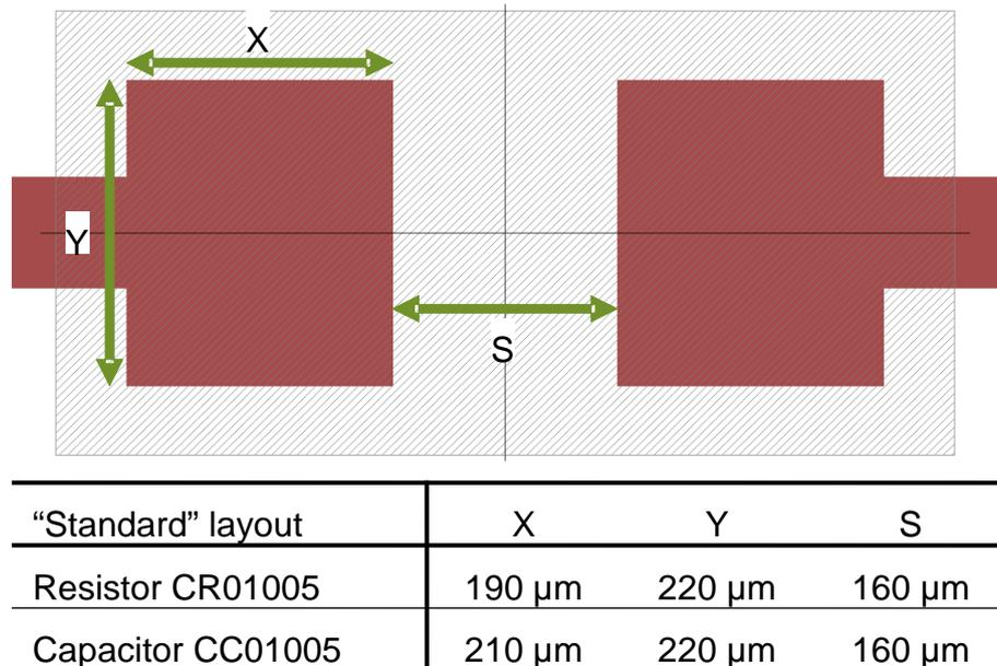
Image 2: A standard design for 01005 components was derived from a number of publications in the literature (cf. [3]).
