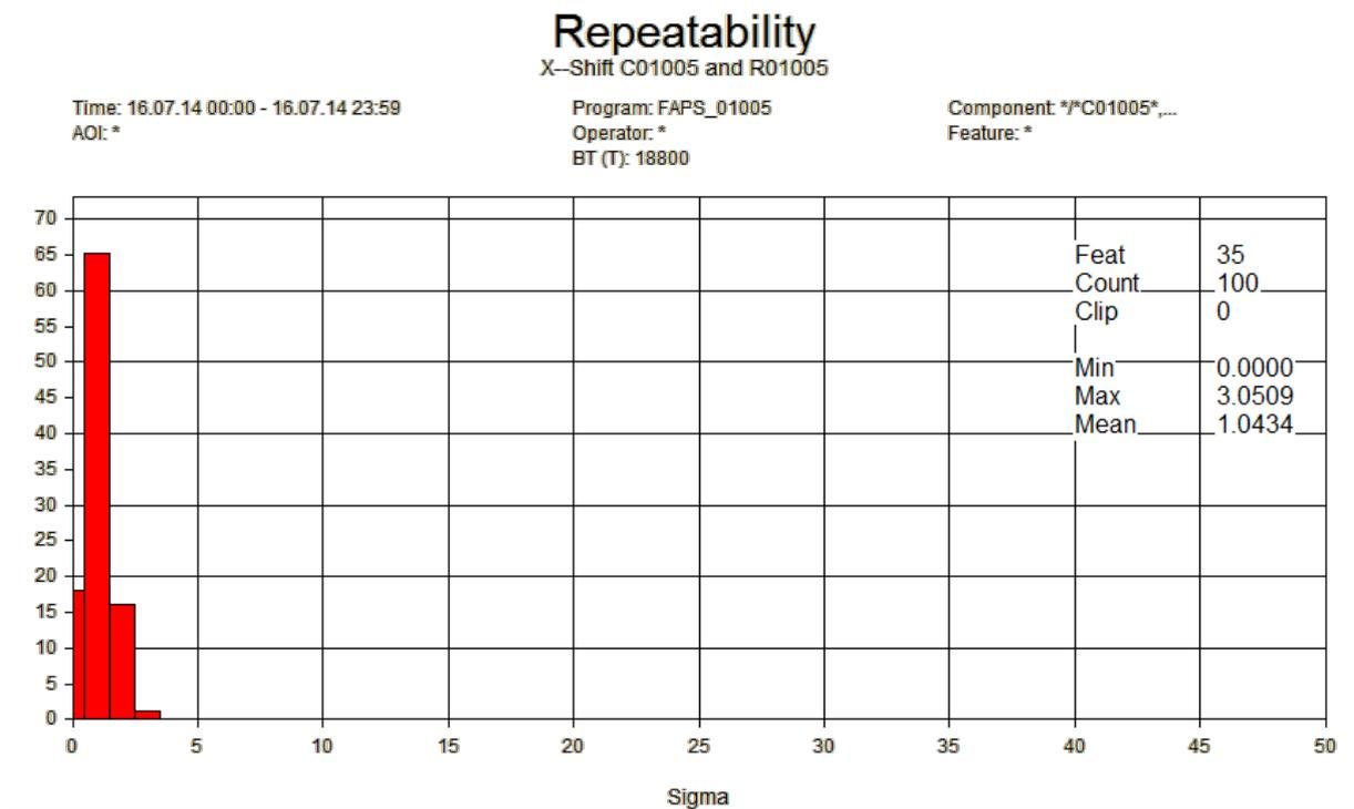
*Image 9: Both the AOI system and the inspection program were examined for stability, measurement capability and reproducibility before the actual measurement.*
