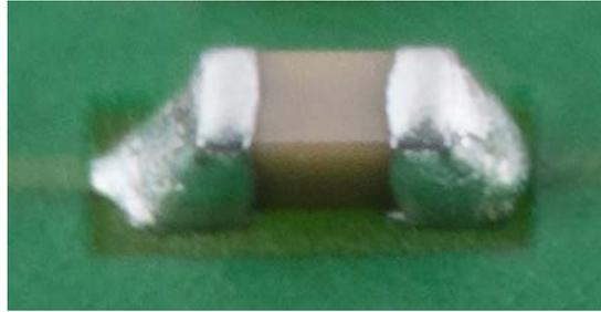
*Image 7: The solder quantity for the CC01005 components is comparatively unremarkable.*
