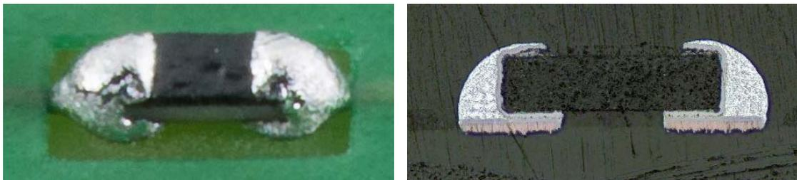
*Image 6: The solder joints display the relatively high solder deposit for resistors (left) and in a typical cross-section (right).*
