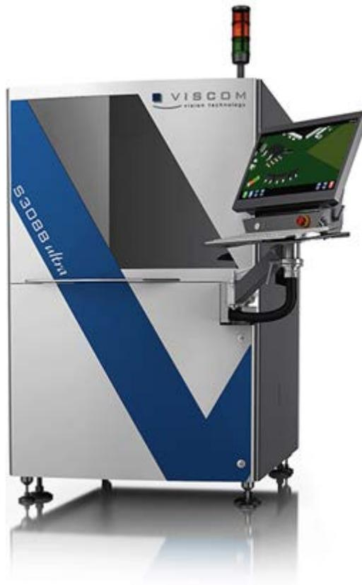
*Image 4: The AOI system S3088 ultra from Viscom AG was employed for measurement of the 01005 components.*
