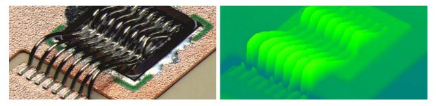
The results of Viscom innovation: 3D wire bond inspection of thick wire on DCB substrate, as a real image and a height image
