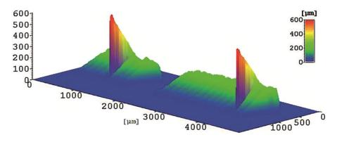
3D information aids not only the inspection of heights and distances. Through the precise determination of the course of the wire, it also enables the inspection of specified wire lengths.
