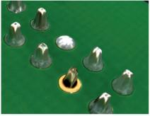
Insufficient wetting (front) and missing pin (back)
