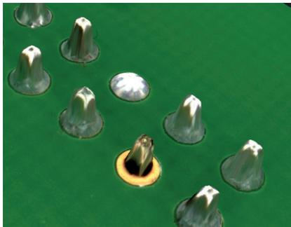
Insufficient wetting (front) and missing pin (back)
