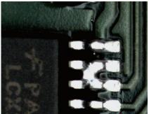
Paste bridge after soldering
