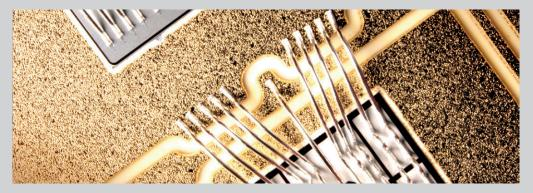
Bonded substrate from power electronics
