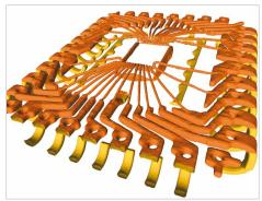
The inspection of a **PLCC** displays the sharp resolution which can be realized with  $\mu$ CT (upper right). **The 25 \mum thick bond wires are just as recognizable as the surrounding die-attach adhesive along the edge of the chip.** In this image, two iso-gray value surfaces were extracted from the volumetric data and separated from each other by color. A  $\mu$ CT investigation, then, always makes sense when it delivers information that is not available in a 2-D image (top left).
