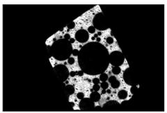
A very convincing example in favor of  $\mu$ CT is that of a 4 mm thick rod from **plaster foam**. In a reconstructed section image (top right), the pores are visible in brilliant clarity, while in a 2-D image (top left), nothing regarding the pores or their position can be determined.
