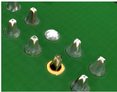
Insufficient wetting (front) and missing pin (back)
