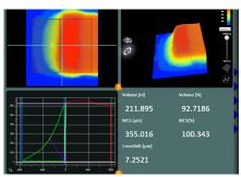
3D solder joint measurement
