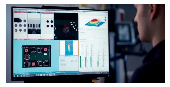
The inspection results of the X8011-III system can be linked and evaluated with images and data from SPI, AOI and AXI for precise defect analysis and process optimization using Viscom Quality Uplink.
