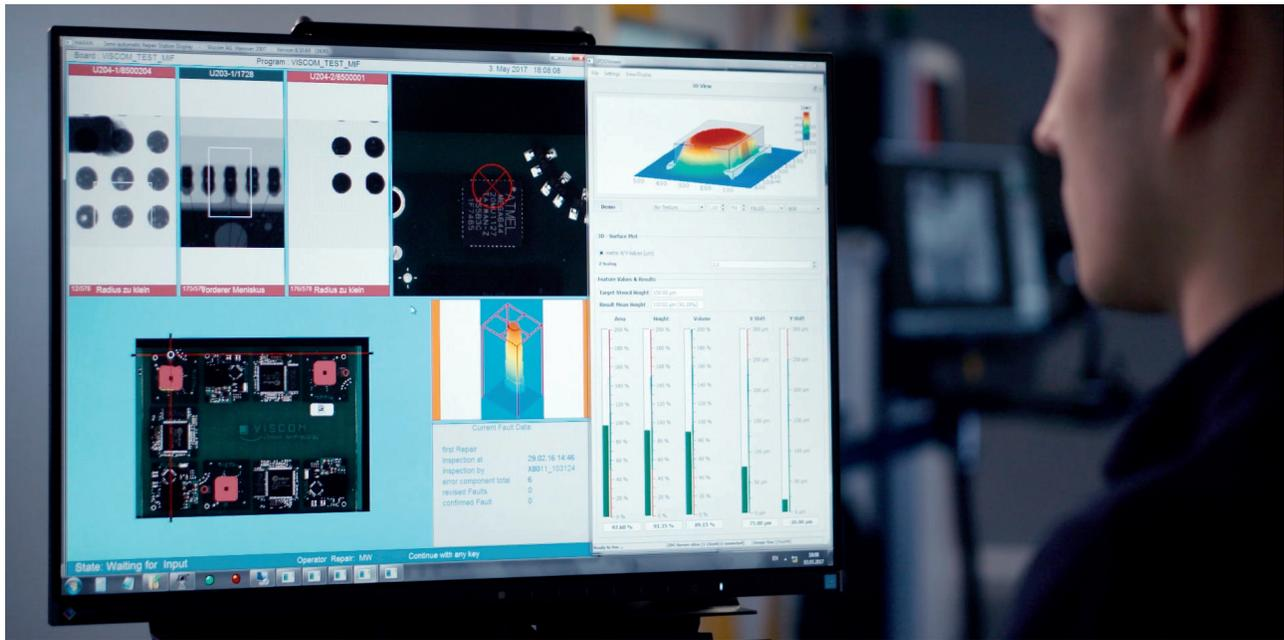
**The inspection results of the X8011-III system can be linked and evaluated with images and data from SPI, AOI and AXI for precise defect analysis and process optimization using Viscom Quality Uplink.**
