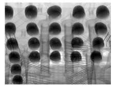
BGA with partially defective solder joints
