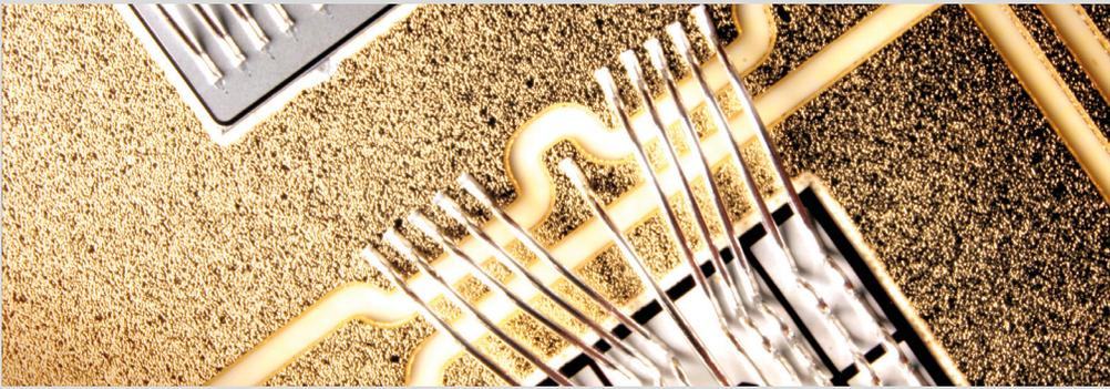
Bonded substrate from power electronics
