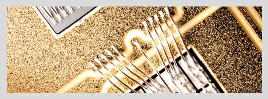
Bonded substrate from power electronics
