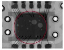
Voids in a surface solder joint
