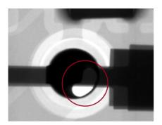
Void in a THT solder joint
