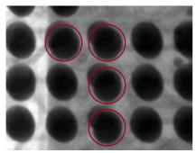
Not connected BGA solder balls
