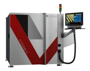
ensure precise inspection of hidden solder joints and components in high-volume production. It is equipped with the xFastFlow transport module, which cuts printed circuit board changing times. With this feature, up to three boards can be processed at the same time. The new handling design also means that significantly larger board sizes can be inspected and the scope of angled radiation is extended.
