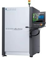
Some of the market-leading features of the S3088 *ultra chrome* include inspection speed of up to 65 cm<sup>2</sup>/s and 65 mega pixels of information in each 50 mm x 50 mm field of view. The resolution is switchable, and with 10  $\mu$ m per pixel even 03015 components can be reliably inspected. Together with the eight angled-view cameras, a virtually shadow-free 3D inspection is one of the key advantages of the system.
