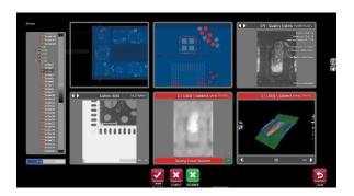
At Viscom's vVerify verification station, 3D MXI inspection results can be compared with those from other inspection gates to optimize the process
