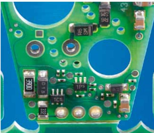
Lead-free ignition electronics with 0201 assemblies
