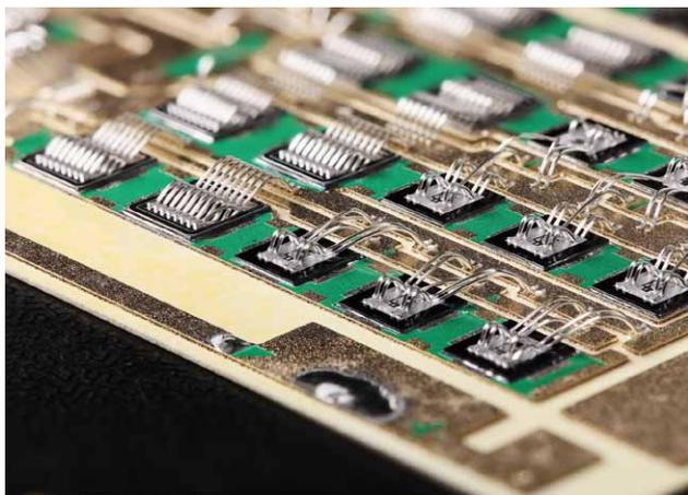
PCB with Wire Bond Connections
