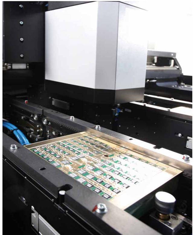
Wire Bond Inspection with Viscom Inspection System S6056BO
