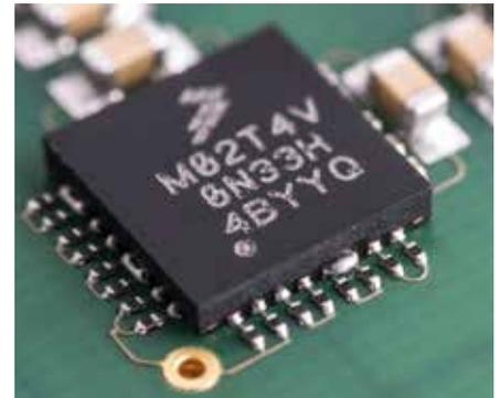
Section of a typical component with hidden soldered connections
