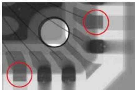
Missing solder on QFN, partial view
