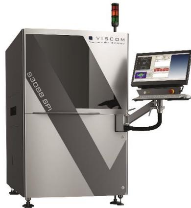
In SMT electronic assembly production, 3D solder paste print inspection has established itself as the additional inspection gate to complement optical or X-ray inspection of electronic assemblies. The key task of the 3D SPI is detecting impermissible printed pads in terms of volume, form, smearing, paste bridges and offset.
